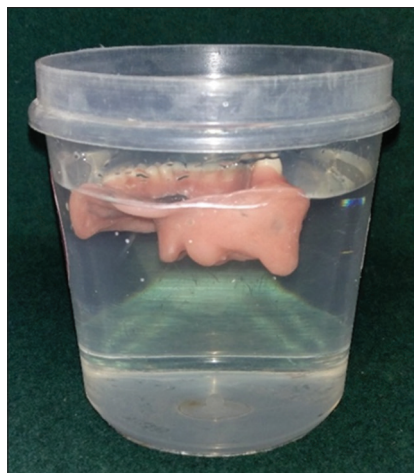
Figure 3: Floating test after making denture hollow
